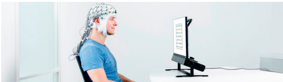
Figure: A participant using a computer equipped with an eye tracker together with electroencephalographic (EEG) equipment. (Courtesy of Tobii Technology.)
